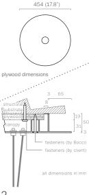
Note: The client is responsible for providing a robust 3/4" (19mm) plywood backing or wood blocking to securely anchor to the structural substrate.
