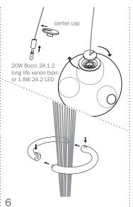
Each pendant terminates in a "headphone jack" type connector, which plugs into a receiving receptacle in the canopy. Plug in each pendant and turn the threaded sheathing into place by hand ensuring that it is adequately tightened. Tools are not required.
