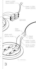
Connect transformers inside the canopy to line voltage. ensuring to match black wire to black wire and white to white. For the ground connection, connect the green wire with yellow stripe to the bare copper wire or green wire in the junction box.
