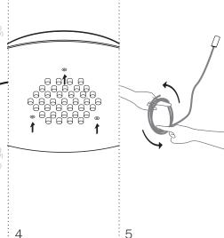
Anchor canopy into the plywood backing using the fasteners provided.
