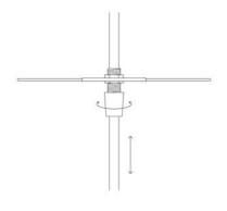
2. Adjust cable length of section within lantern to locate lamp/ bulb holder into central position. Hand-tighten clamp to fix cable.
