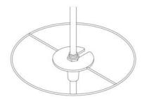
1. Slot cable into top plate of Hotaru lantern and hand-tighten fixing nut.
