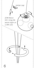
Bocci 24.1.2 long life bipin xenon lamps included. Plug the lamp into the socket. Do not touch the lamp with your bare hands.
