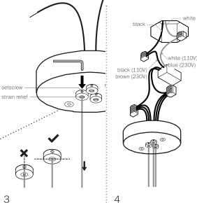
Connect the coaxial cable to the open slots in the terminal block on the 12V side of the transformers. Ensure that the braided outer wires are all connected to one 12V output wire and all inner insulated wires are connected to the other or a short will occur.
