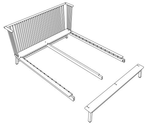
b) Insert a Universal Connector into the rebate in the footboard end of one sidebeam, and place a metal dowel into the corresponding pre-drilled hole in the footboard. Guide the metal dowel into the Universal Connector and tighten firmly with an Allen Key. Repeat this procedure for the second sidebeam.
