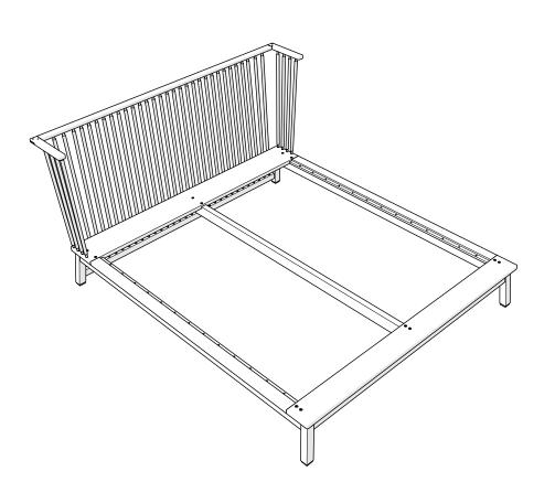
d) Insert 2x M8x30 bolts into the footboard at each connection point and tighten with an Allen Key.
