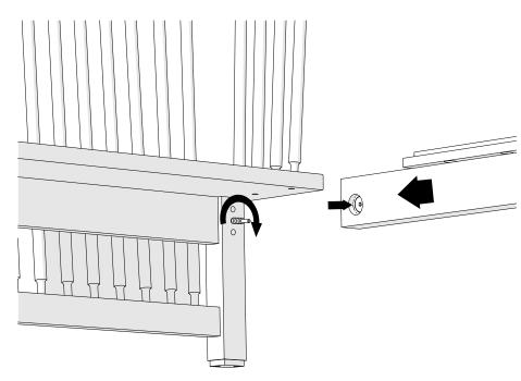
e) Insert 2x  $\rm M8x30$  bolts into the headboard base at each connection point and tighten with an Allen Key.
