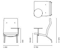
**Dimensions** L650 x D790 x H1070mm Weight 25kg Design: 2020
