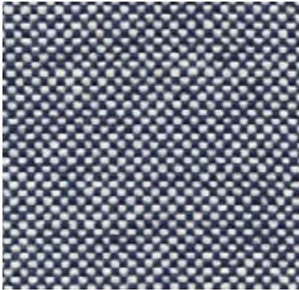
Hopsak is an expressive, flat plain-weave fabric made of polyamide. The duotone colours offer a multitude of design possibilities in high-contrast, brightly hued or subtle combinations of warp and weft threads. Highly durable and robust, Hopsak can be used in private interiors as well as public areas.
